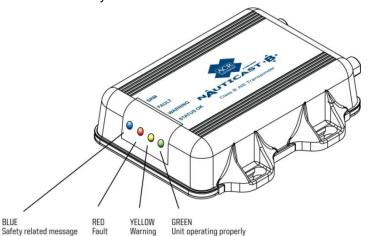
If the red LED illuminates continuously, the unit should be assumed to be faulty. It should either be switched off (power removed) or, if this is not practical, any other vessel position information derived from the unit should not be used. It should also be assumed that the unit is not transmitting valid position information for your vessel.
