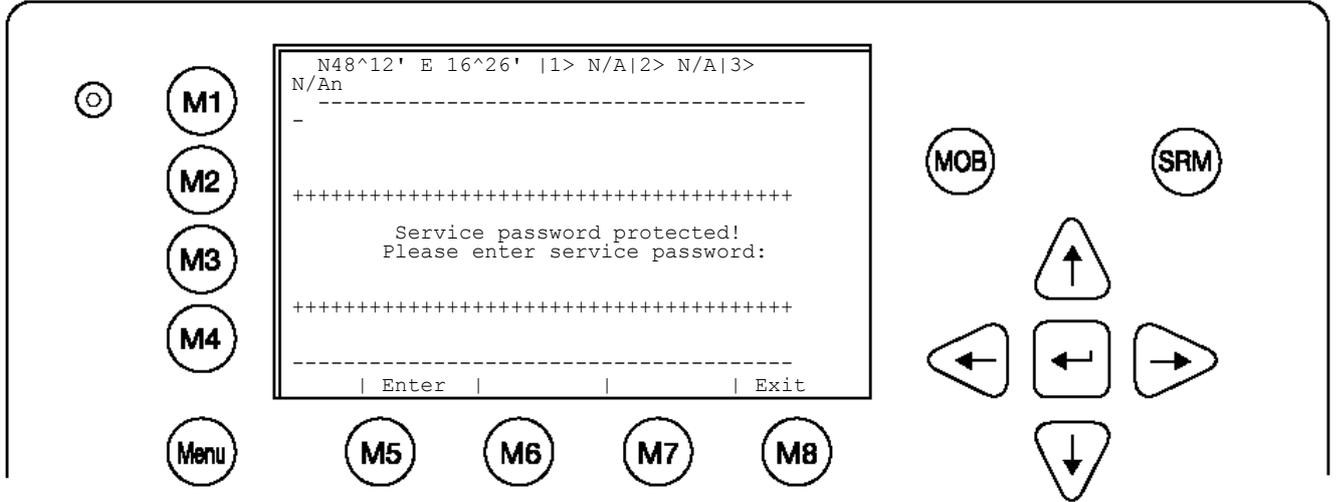
Select Submenu 1 "Change Service Password" with cursor button [Up] & [Down] by pressing Number 1 on the keyboard.
