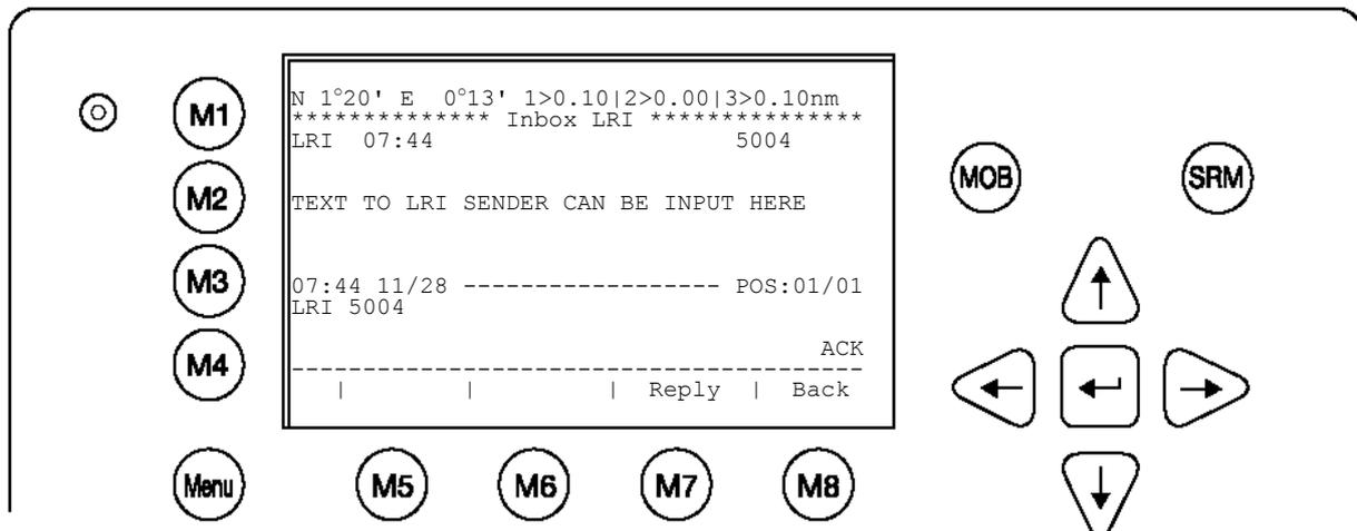
An LRI has arrived; the NAUTICAST™ Settings are configured to **Manual Mode**:
