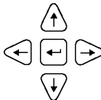
In addition to the actually displayed [Enter] button, the center of the cursor cross always has the Enter functionality.
