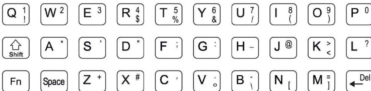
Tip: The NAUTICAST™ automatically changes the keys “Q” through to “P” to numerical input when the current application requires numbers, rather than letters to be input. This feature is enabled when [NUM] appears on the bottom left hand side of the screen.
