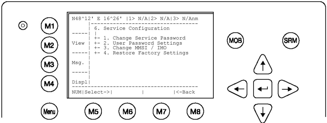
Select Submenu 1 “Change User Password” with cursor button [Up] & [Down] by pressing Number 1 on the keyboard.
