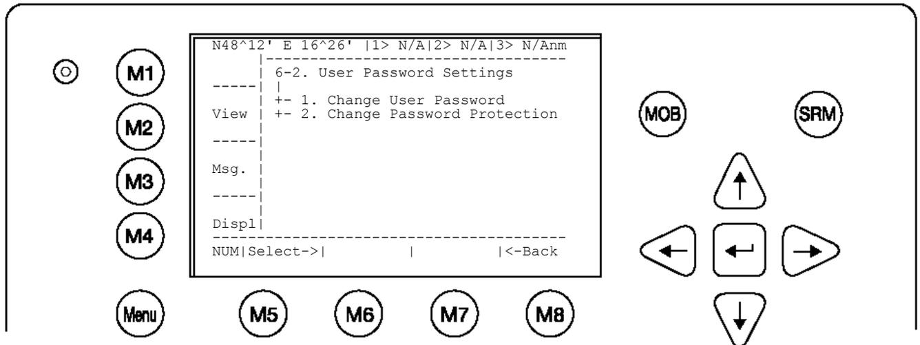
Enter the new Password. A minimum of 6, a maximum of 8 characters are allowed. Should the new password include numbers, use the shift key to generate them.
